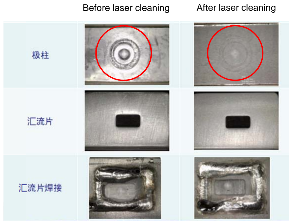
Before & After laser cleaning
