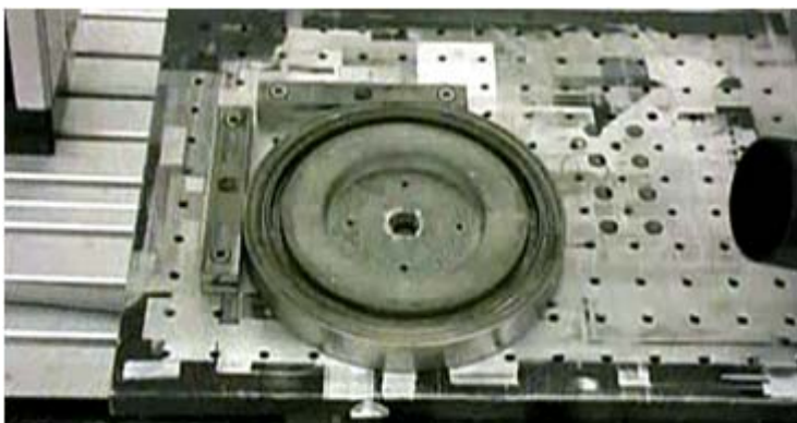
Remove the residue of the titanium nitride coating mold
